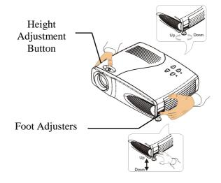
Adjust the projector angle using the Height Adjustment Buttons.
